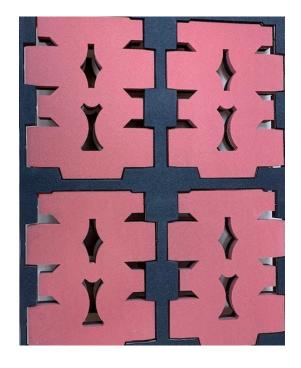
Holding down the sheet during the blanking process is key. If a sheet has narrow sides of scrap; a standard straight hold-down bar may not be enough to hold the entire scrap down while the blanking process is done on today's high speed blankers. When you have a double cut layout Sharples Steady Blanker will assist with holding the entire web while the upper and lower blankers do their jobs.
